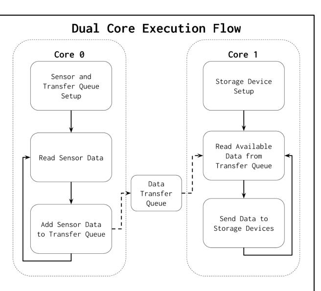
**Parallel Computing:** Utilizing the RP2040's dual ARM Cortex-M0+ cores, the flight software splits tasks to be completed in parallel (see above).
