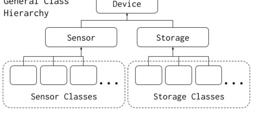
The flight software is designed to be **modular**, allowing it be modified easily between payload iterations. Peripherals are abstracted, inheriting from a parent class that allows each to be managed identically despite implementation differences.
